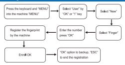
Note: when choosing a password or ID card (machine with the function),the name of the person can be uploaded through the access control software;
